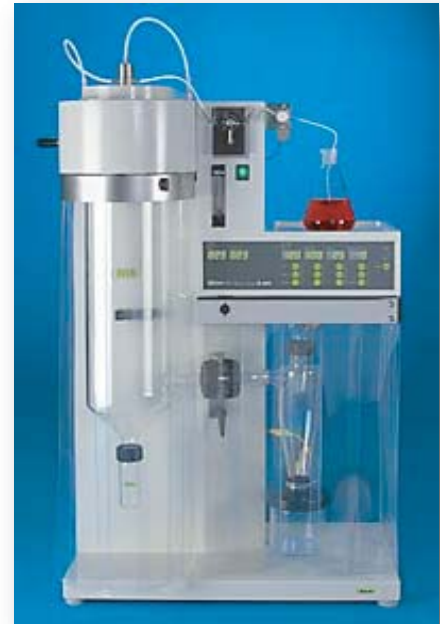
Figure 1. Büchi B-290 Spray Dryer
