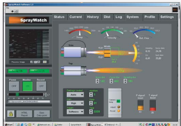
Fig. 3. The feedback to the operator: particle temperature, velocity and flux
